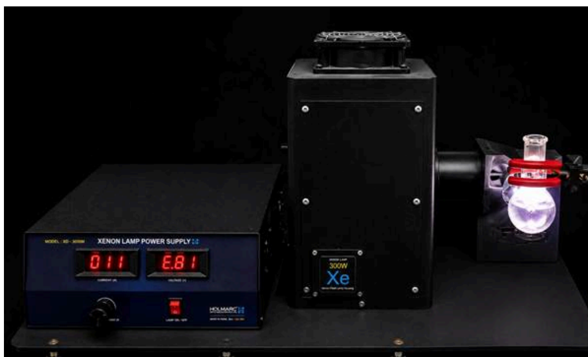
Fig: Experimental setup for photocatalysis consisting of the irradiation source and the reaction medium.
