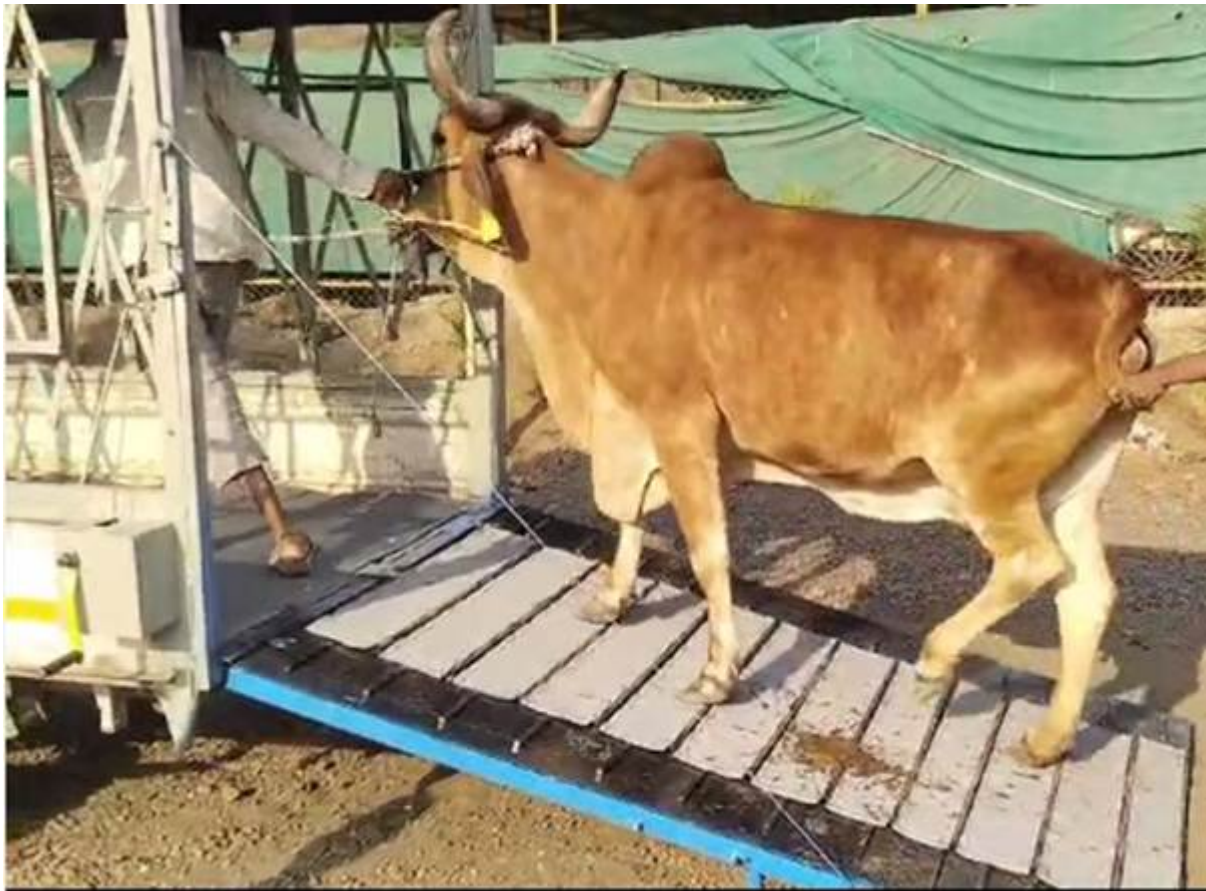
Fig 2: Modular Cage with adjustable ramp for ease of loading and unloading as per the specified guidelines obtained from the user
